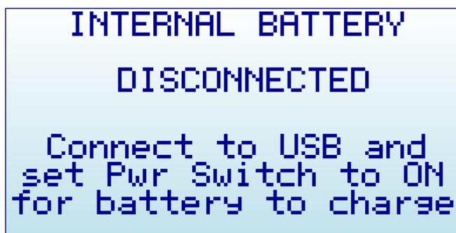
As soon as the power switch is set to the correct position, the screen will display correct charging status.
