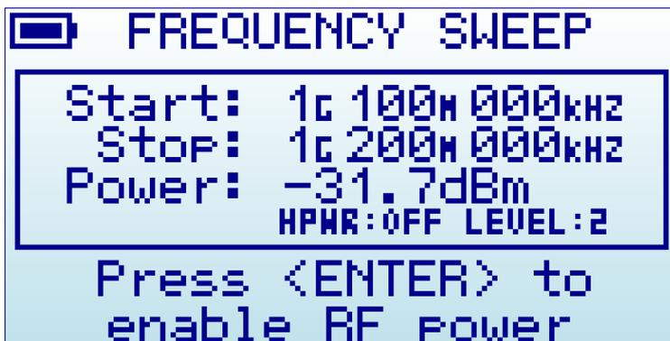
To start the Frequency Sweep, press ENTER key. The Sweep will be active until ENTER is pressed again.
