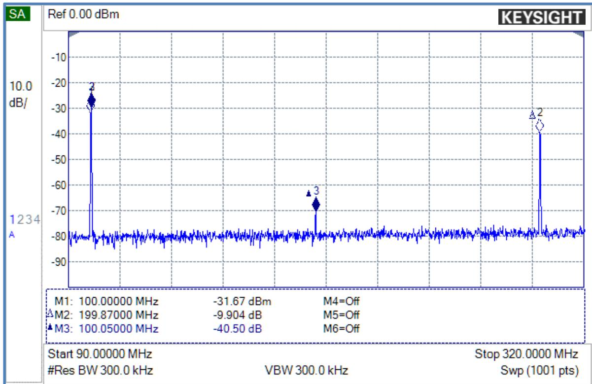
Image above: 100MHz 2<sup>nd</sup> (-40dBc) and 3<sup>rd</sup> (-10dBc) Harmonic using baseline RFE6GEN model
