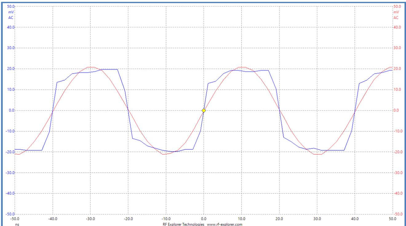
An example at CW 100MHz shows dramatic reduction of 2<sup>nd</sup> and 3<sup>rd</sup> harmonics:
