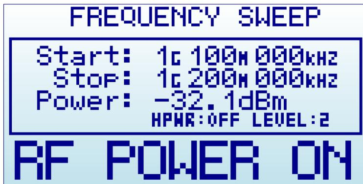
In above example, Frequency Start is 1,100.000MHz and Frequency Stop is 1,200.000MHz. The nominal power level is -31.7dBm with *High Power:OFF* and *Level:2*. Using UP and DOWN button will change power level one step at a time.
