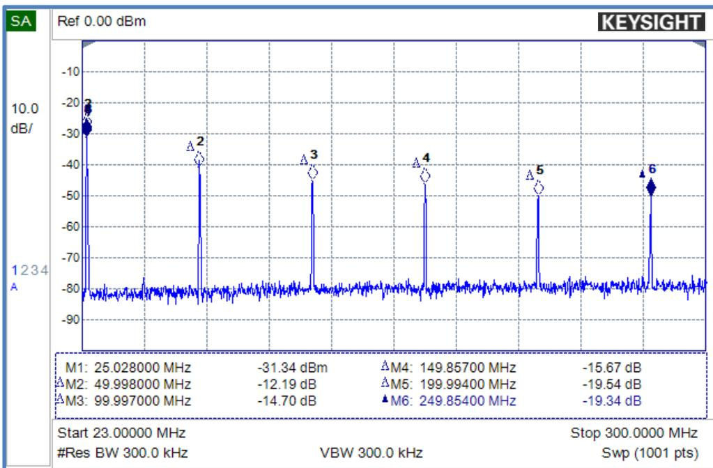
Example output signal including harmonics from a 25MHz CW signal in RFE6GEN baseline model.
