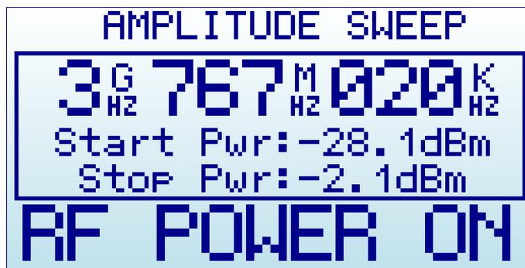
Using LEFT and RIGHT buttons the frequency can be decremented/incremented manually, as well as using the Frequency Menu where Step Delay is also configurable.
