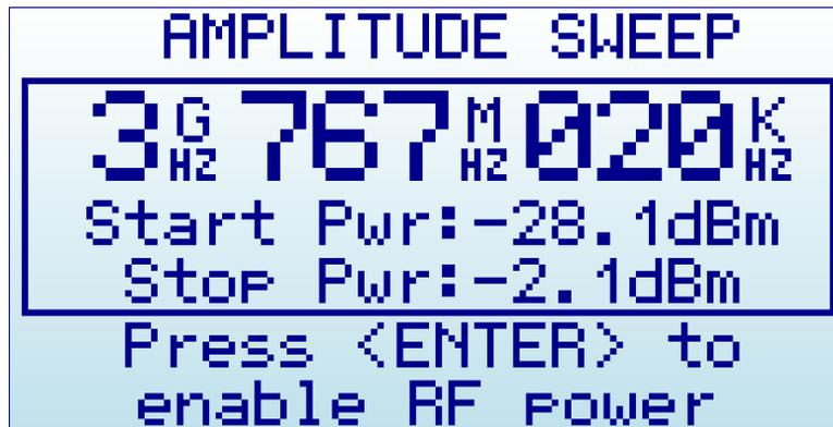
To start the Amplitude Sweep, press ENTER key. The Sweep will be active until ENTER is pressed again.
