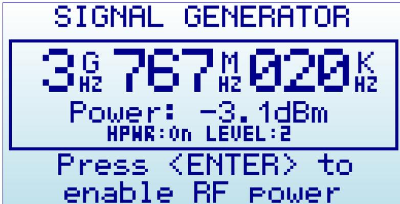
All elements on screen are important parameters to understand how the Signal Generator is working at any given time. In the baseline model (non Combo) model the power level is one of the possible 8 selectable values from Menu.
