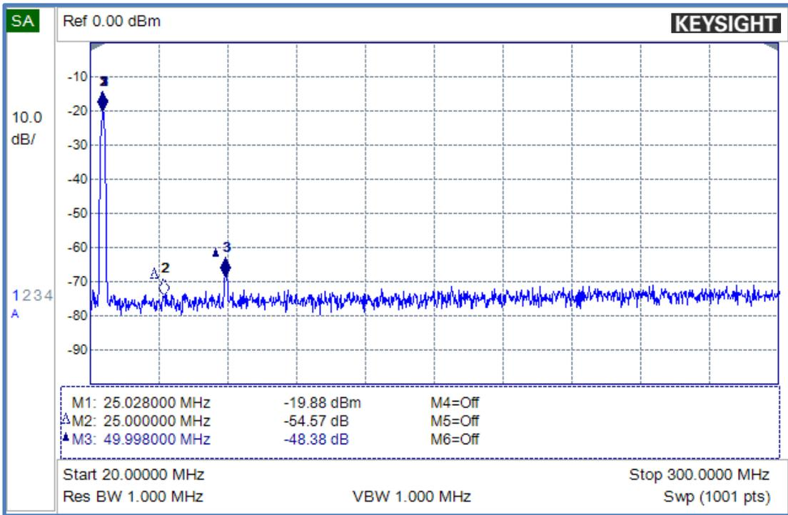
Example output signal including harmonics from a 25MHz CW signal in Combo filtered model with significant improvement over baseline model.
