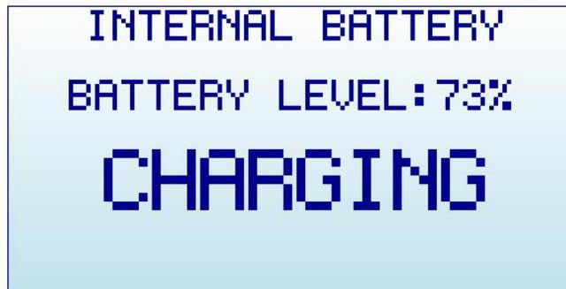
At this point you can close this screen pressing ENTER or RETURN. If you keep it active for more than 15 seconds, it automatically sets the device in SLEEP MODE - all internal circuits and LCD backlight go off, except for charging and minimal CPU monitoring - This is the recommended procedure to charge the device overnight. Note: for the sake of clarity, below black/white screen images are depicted when LCD backlight is OFF.
