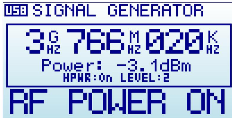
Please note standard precaution of RF power delivered without a connected load.
